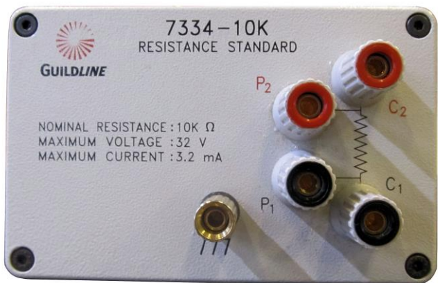
Figure 3-3: 7334 Series from 1 Ω to 10 kΩ
