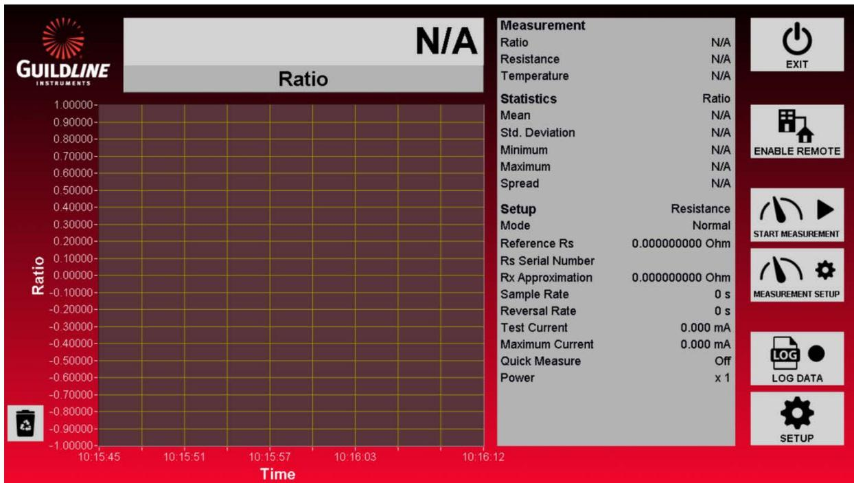
The data on the graph can be cleared by touching the “Trash Bin” icon to the bottom left of the screen. Note that clearing the graph does not remove the data from the stored data if “Log Data” is enabled. Also note that the statistics will be cleared as well. These statistics reflect all the present data in the graph.
