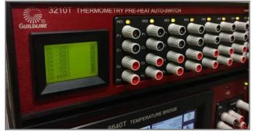
single or multiple tests can be initiated while the Bridge is unattended. All user **definable test variables**, such as excitation current, pre-heat current, measurement speed, reversal rate etc. can be **programmed on a per test basis**, giving the **users full control and flexibility** in conducting well designed measurements, and for calibrating temperature probes.
