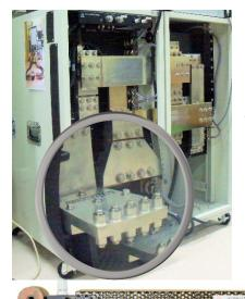
**How good is the 6623A-PCS?** Measurement results from a 1000 Ampere Intercomparison of two NMIs (Test Results shown below right) came within 5 ppm of each other. One setup was a Guildline 6623A-PCS/4000A System with our 66259 Controller. This system is shown to the left.
