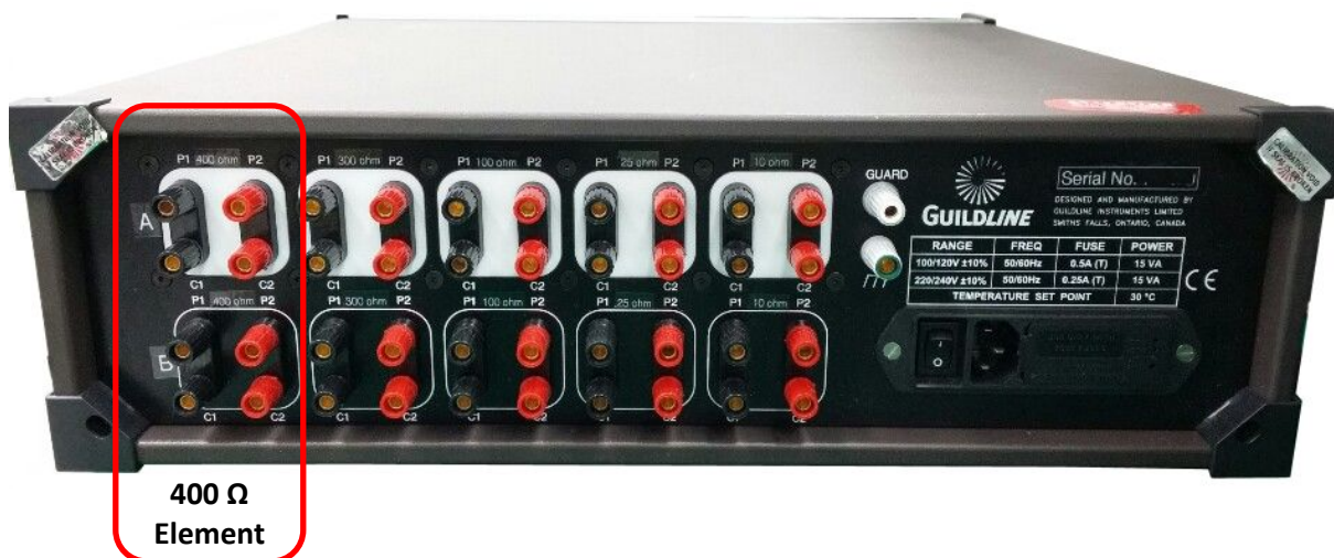
Model 7334-TC with 10 Custom Elements in a Temperature Controlled (TC) Enclosure
