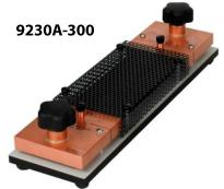
For models from 300 A to 500 A, Guildline utilizes higher power copper current input terminals and also uses a custom alloy for the resistive material. The number one selling model in this design is our 9230A-300 shown to the left. Like all Guildline Shunts, notice the circular current connections and precision cut-outs to channel the current allowing for the best in repeatability and stability for current measurements.
