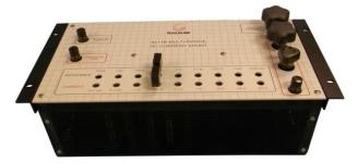
A. The unit consists of nine shunts with a 4-terminal configuration. The design optimizes a number of important factors such as the effects of self-heating, size, weight, ease of operation and wide measuring range. The 9211A provides a wide range precise current measuring capability when used with a potentiometer or digital voltmeter as a readout.
