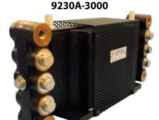
The Model 9230A- 3000, with a 10  $\mu\Omega$  resistance value, is specified for currents up to 1500 A with natural air convection and up to 3000 A with the 92310 forced air unit. However the 9320A-3000, like all Guildline shunts, can be used up to full rated current in ambient air. The 9230A-3000 has 11 connections points at both ends, with a symmetrical pattern, and stainless steel helicoil inserts.
