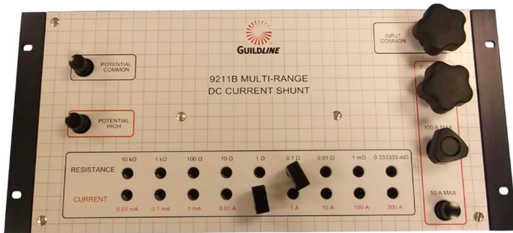
Figure 3-1 : 9211B Current Terminal Connections
