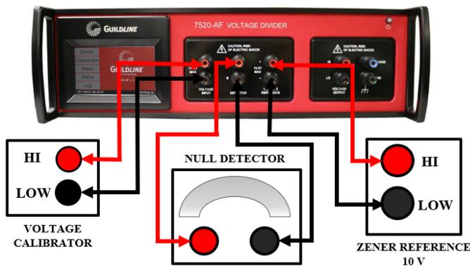
Before starting a measurement, zero the DMM/ND as per the Operator Manual of the instrument you are using. In case of using a DMM as a ND, set the parameters of the DMM for an optimal measurement.
