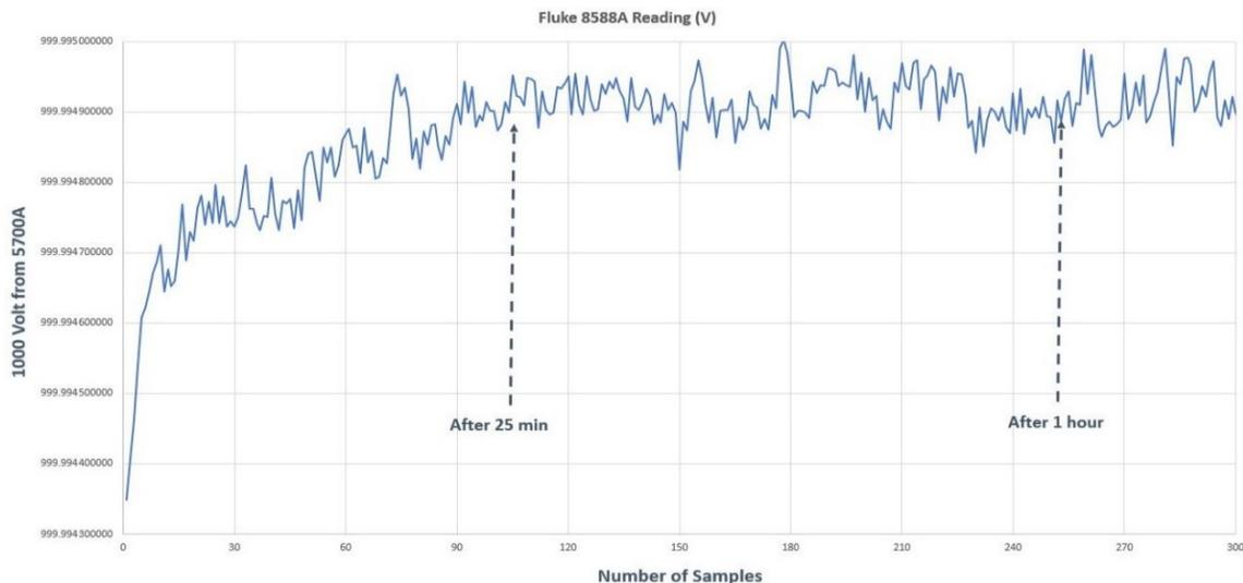
network to stabilize. For input voltages less than 20 V self-heating is not material. For input voltages between 20 V and 100 V it is recommended that a wait time of 10 minutes be used. For input voltages between 100 V and 1100 V it is recommended that a wait time of 20 minutes be used. However, if using a calibrator to generate the input voltage an equivalent time is required for the calibrator's output voltage to stabilize as illustrated at the bottom of the previous page.
