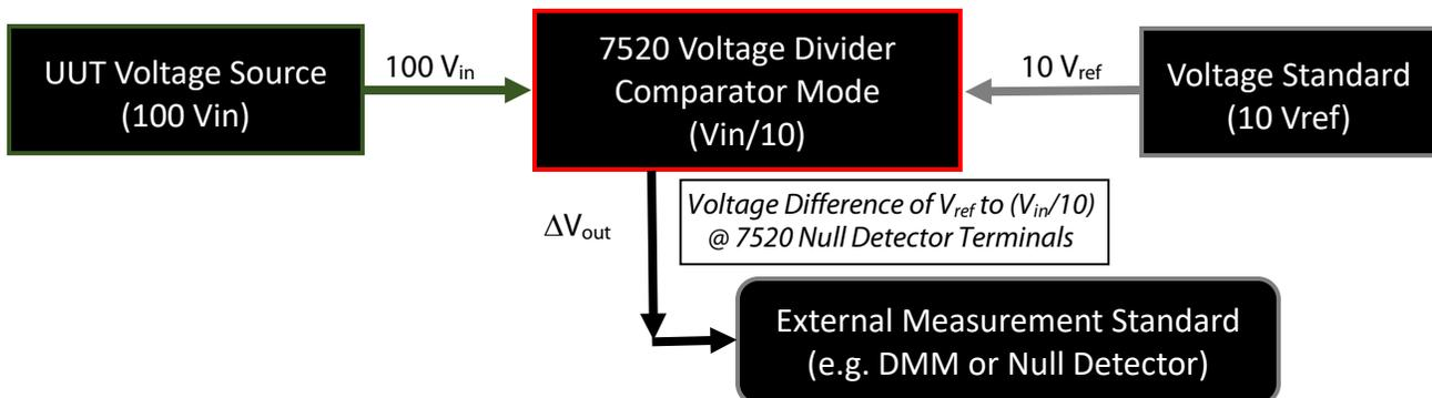
In addition, when operated in the Comparator mode of operation, the polarity of the Voltage Reference can be switched inside the 7520 manually or automatically. This enables fully automated polarity switching, and thus a fully automated calibration because the wires connecting the Voltage reference do NOT have to be manually switched to change the polarity. This also speeds up the calibration process because there is no wait time required due to switching the Voltage reference leads.
