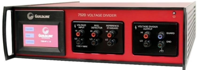
Special care has been taken to minimize thermal offsets and noise during use, and during the 7520 self-alignment/self-calibration. The voltage reference, resistive voltage divider networks, and optical null detector are all inside a thermally regulated and EMI shielded chamber. The ultra-low thermal switches used are high isolation relays. In addition, the use of a newly designed optical null detector guarantees high isolation and low noise during the self-alignment process.
