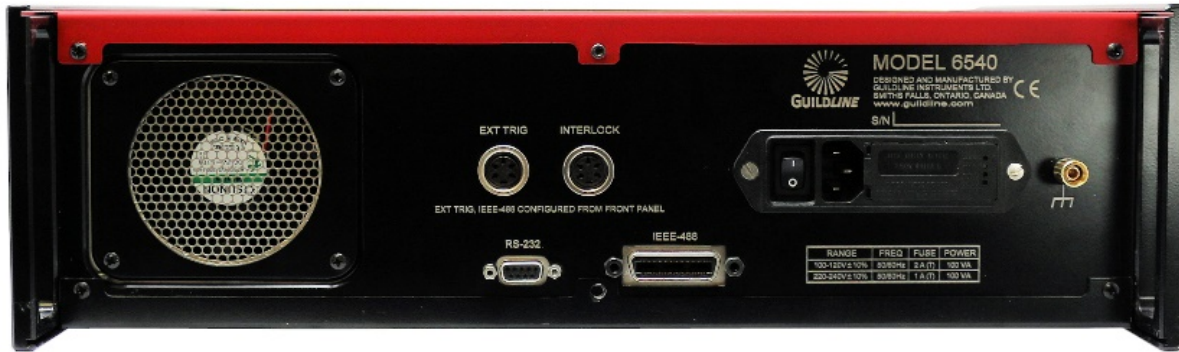
Figure 2-4: 6540 Rear Panel Connectors
