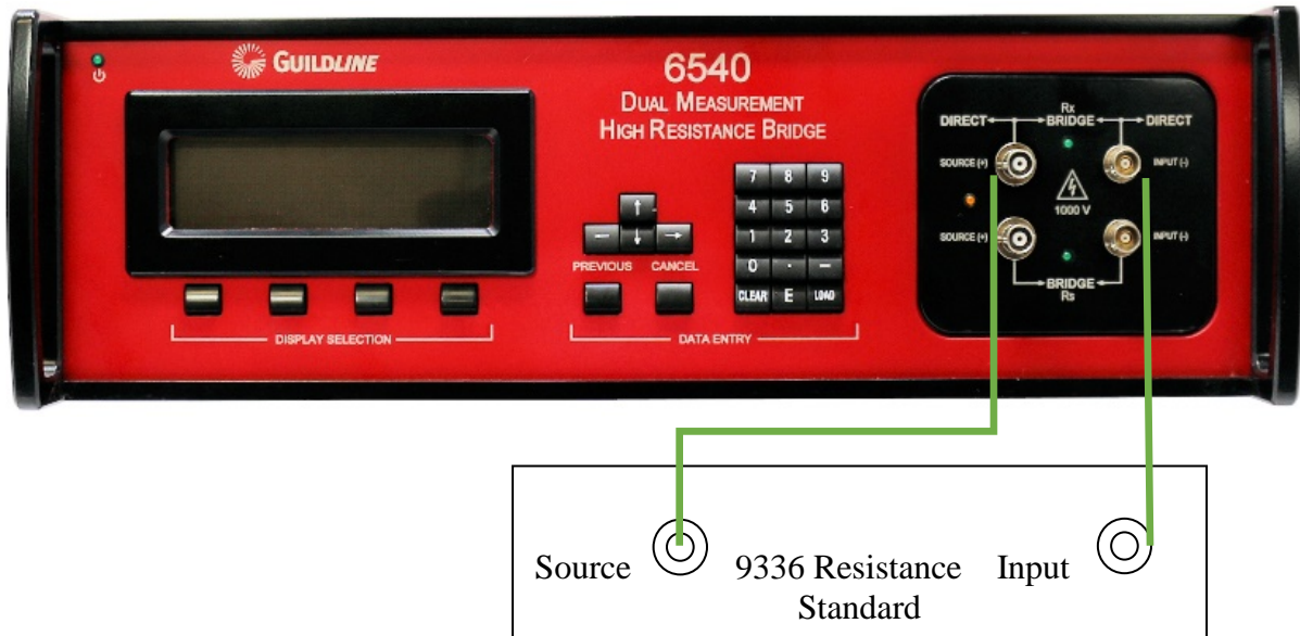
Figure 2-3: 6540 Front Panel Connectors – Direct Mode
