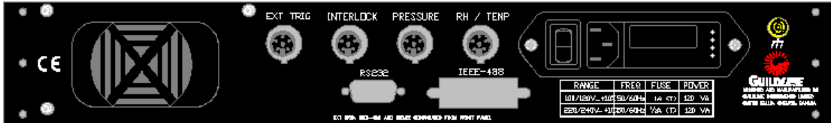
Figure 2-4: 6530 Rear Panel Connectors
