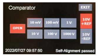
In addition, the 7520 is the only voltage divider where the polarity of the Voltage Reference can be switched inside the 7520 manually or automatically. This enables automated polarity switching for the Voltage Reference, thus the wires connecting the Voltage reference do NOT have to be manually switched to change the polarity. This also speeds up the calibration process because there is no wait time required due to switching the Voltage Reference leads.
