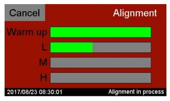
uncertainties. The self-alignment process can be initiated through the front panel or a SCPI command and takes about 2 hours to complete. Once performed, the self-alignment is good for one month. The process can be run at any time, such as at the end of the day or over the weekend.
