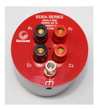
**GUILDLINE INSTRUMENTS 9330A SERIES** of Oil Based DC Resistance Standards are designed for high accuracy resistance calibration in oil (i.e. fluid baths) or in air. They range in ohmic value from 0.001  $\Omega$  to 10 M $\Omega$ .
