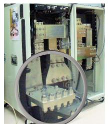
**How good is the 6623A-PCS?** Measurement results from a 1000 Ampere Intercomparison of two NMIs (Test Results shown below right) came within 5 ppm of each other. One setup was a Guildline 6623A-PCS/4000A System with our 66259 Controller. This system is shown to the left.
