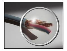
In looking at a cross section of the SCW Wire, you will find the highest possible build quality of any measurement wire. All Guildline SCW wires consist of a pair of either 18 or 22 Gauge solid copper conductors packaged in a low density polyethylene insulation (color coded) (1), with a clear low density polyethylene inner jacket (2), surrounded by a bare copper braid shield (3) with a (mylar or polyester separator (4), and an oil resistance protective grey PVC outer jacket (5).
